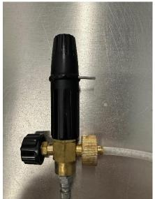
Remove the black sleeve, from there you will have access to the components of the foam cannon. Remove the small clear pickup hose from the assembly, it may help to place the brass assembly in a vice to hold your components as you remove them. Using your crescent wrench, remove the brass cover piece circled below.
