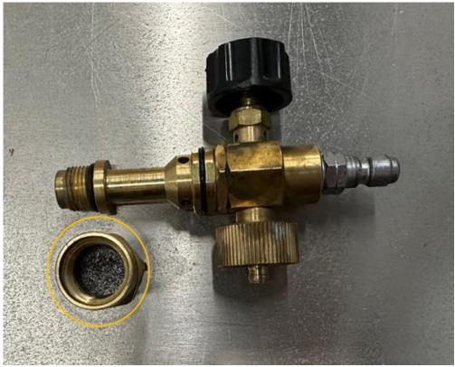
If it feels like it is taking too much pressure to remove, try adding warm water or vinegar into the assembly, it will help loosen the filter. It can get stuck from a result of soaps that may have wax in them for example.
